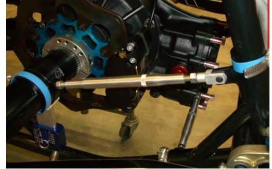
TRU-SQUARE tool attached to a sprint car chassis to illustrate the proper installation.
